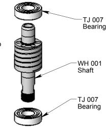
4. If you have a Fill Tube (TJ 064), insert it thru the Shaft Seal in the Body up to it's shoulder. Pour Viscous Fluid into the Body about 1" deep. Insert the Shaft into the Body, allowing the Shaft to push out the Fill Tube. If you do not have the Fill Tube, insert the Shaft into the Body and pour viscous fluid into the Body; allow the fluid to settle down thru the top bearing and around the Shaft and keep adding fluid until it covers the top bearing. It will take about 10 minutes to get
